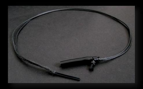
Slim Shim (spring metal) for single locked handcuffs. Slides inside silicone tube and doubles as break away retainer for neck carry.
